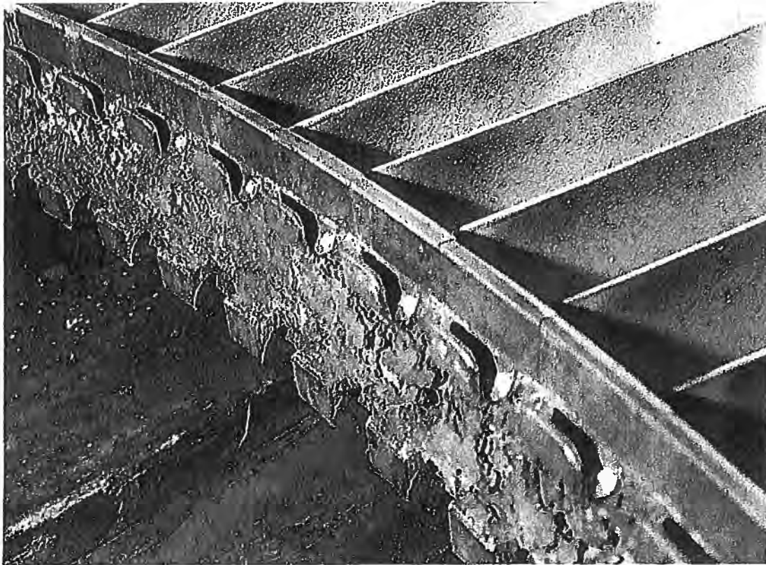
View of 7th Stage OGV Ring showing worn inner vane feet
