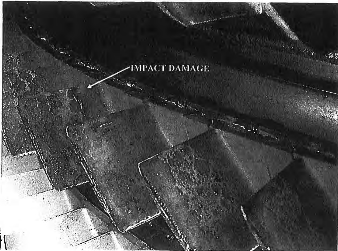
View of 5th Stage HP Compressor Blades showing impact damage
