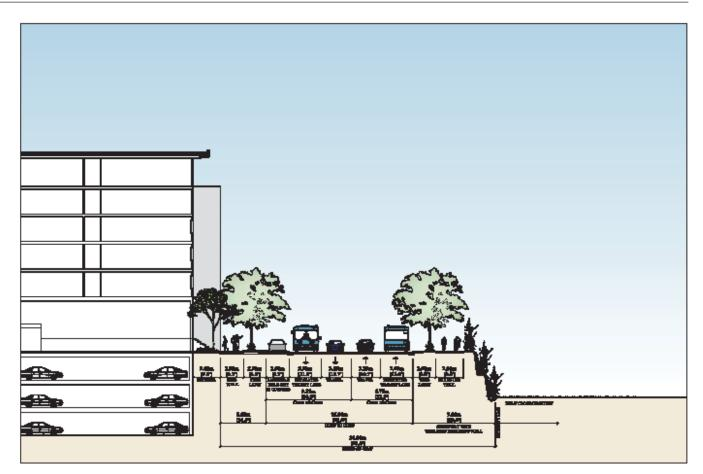
BOULEVARD RAMPING AT CNR - 30 meter R.O.W. (Section Scale 1 : 3)
