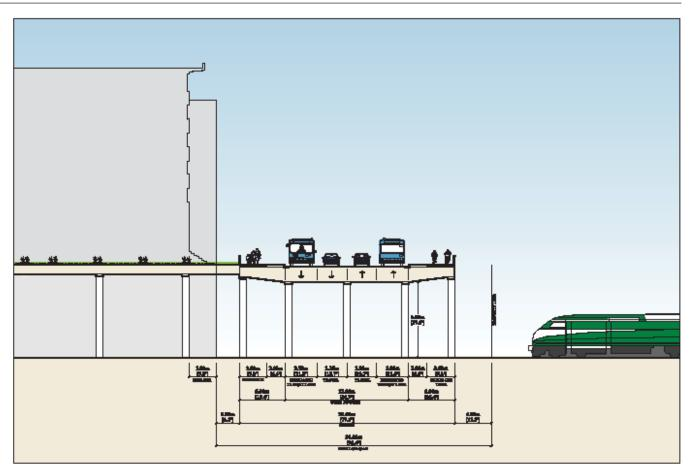
BOULEVARD BRIDGE - 23.5 meter wide bridge and 30 meter R.O.W. (Section Scale 1 : 3)
