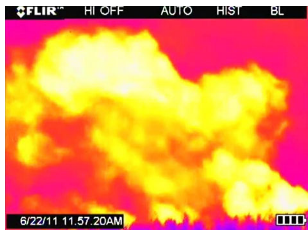
Fig. 1 Venting of natural gas into the atmosphere at the time of well completion and flowback following hydraulic fracturing of a well in Susquehanna County, PA, on June 22, 2011. Note that this gas is being vented, not flared or burned, and the color of the image is to enhance the IR image of this methane-tuned FLIR imagery. The full video of this event is available at http://www.psehealthyenergy.org/resources/view/198782 . Video provided courtesy of Frank Finan
