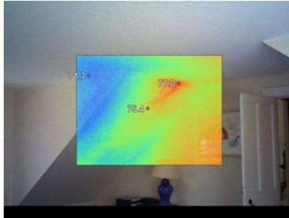
**Figure 22. Temperature Differential in a Closed Structure (B)**
