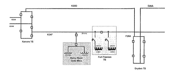
Figure1: Single Line diagram of the system
