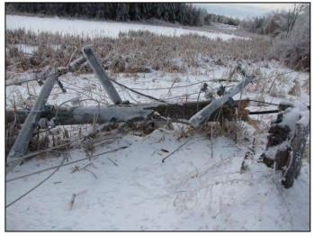
A 44 kV M-class feeder pole in Brockville that broke during the ice storm.
