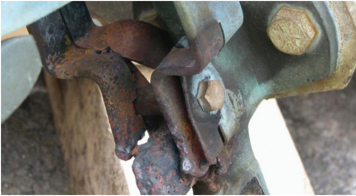
Severely corroded switch blade.
