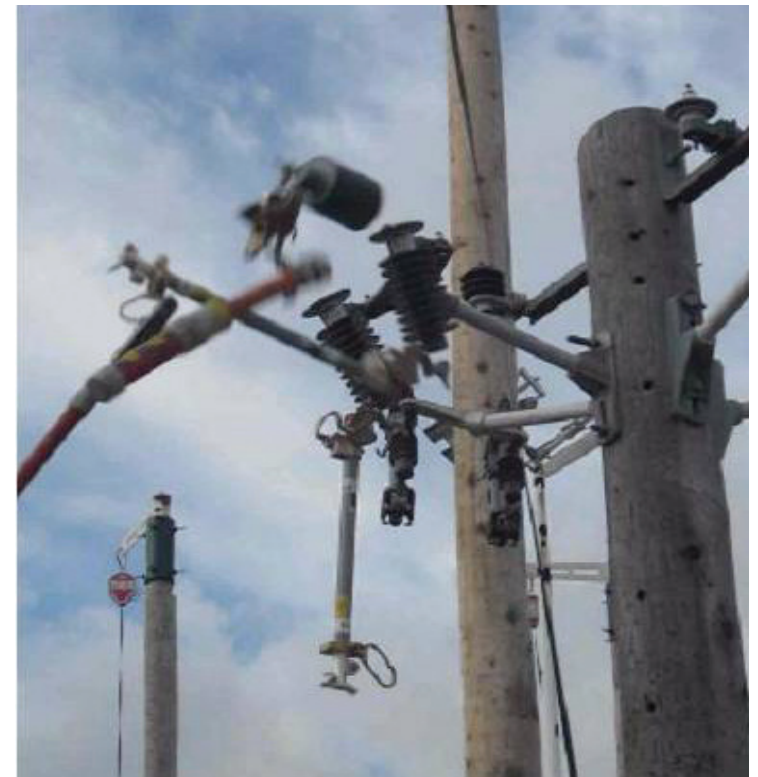
Failure after switch operation during testing.
