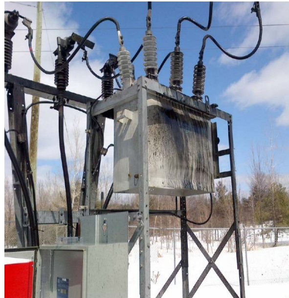
Figure 13 - Bridlewood Recloser Exploded Internally
