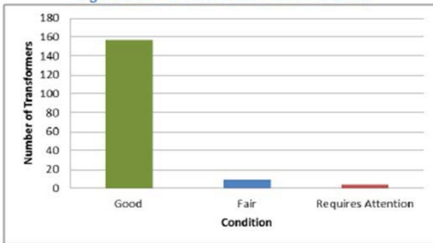
Figure 2.2.9 - Station Transformer Condition
