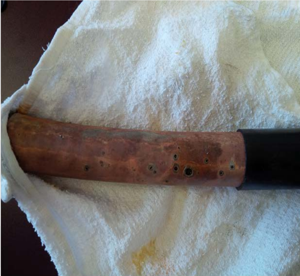
Faulty 44kV PILC Cable removed from Riser Pole at a Substation – pitting of the lead sheath
