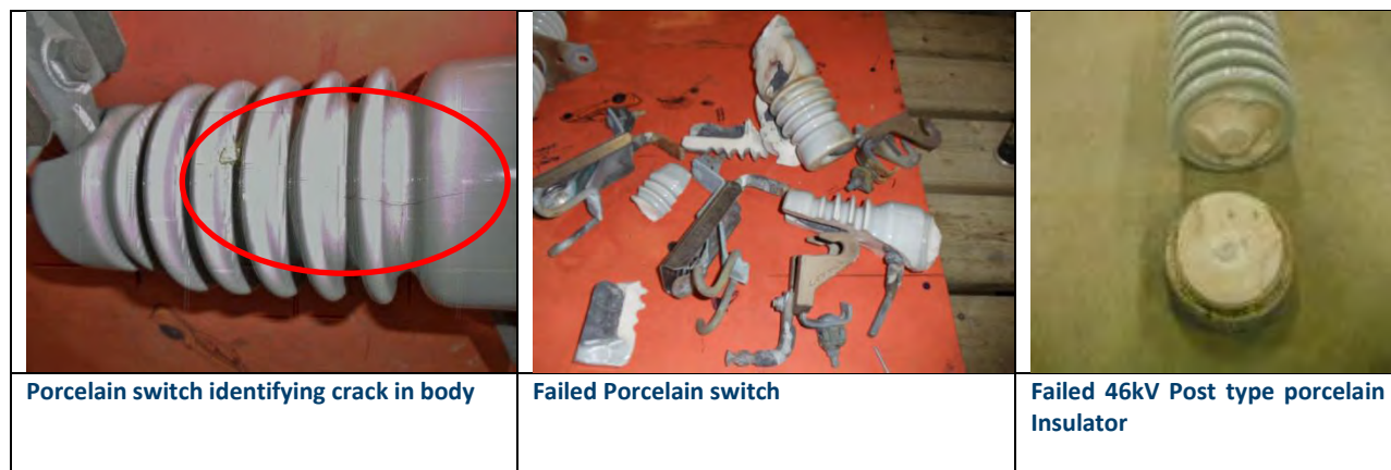
Figure 26 Examples of Failed Porcelain Equipment
