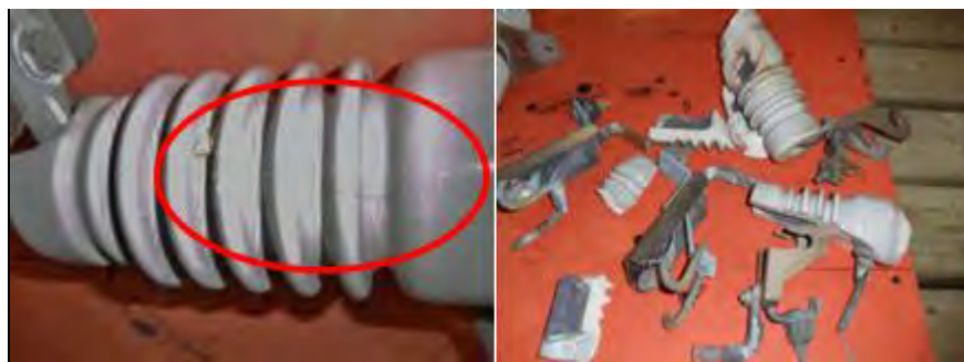
Figure 3-15 Cracked Porcelain Insulator (left), Broken Porcelain Switch (right)
