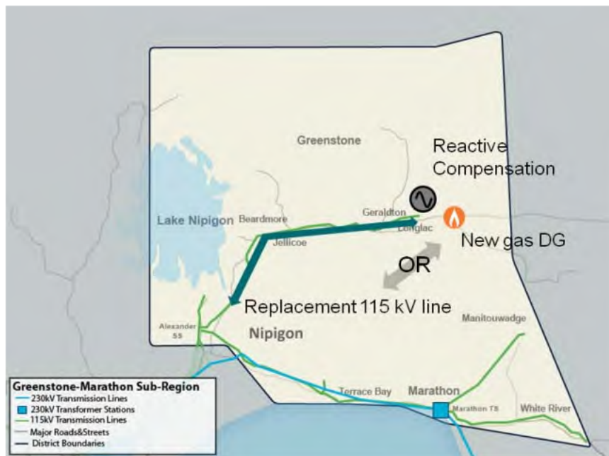
Figure 9-2: Recommended Stages 1 and 2b
