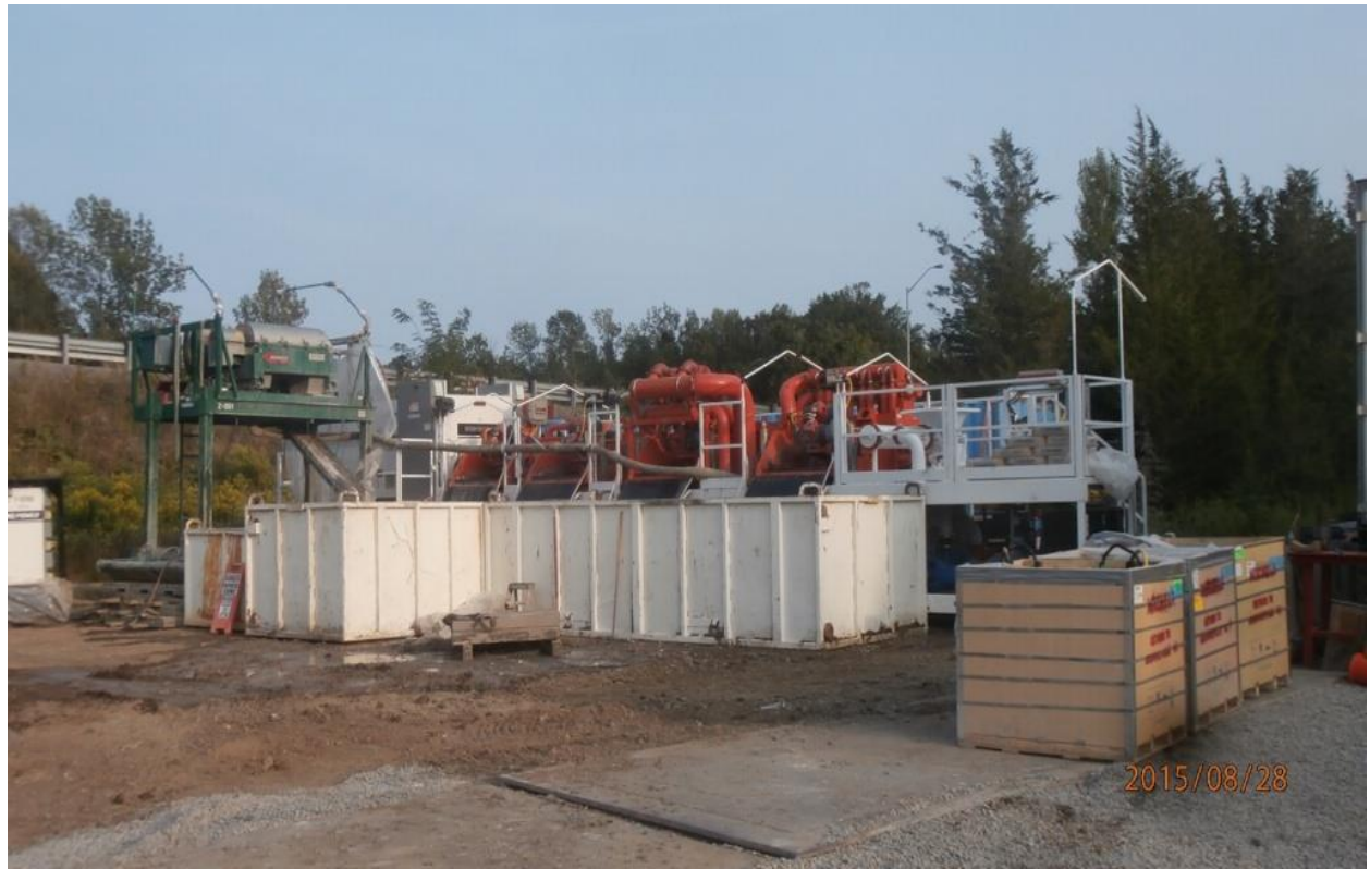
This view of the drilling operation shows the mud tanks and shakers where the rock is separated from the mud so the mud can be recycled back through the drill rod.
