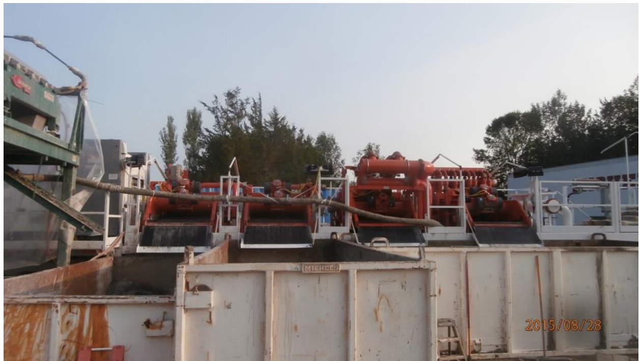
A close up view of the shakers. The first shaker removes the larger rocks/cuttings with the process continuing until the very fine rocks are removed leaving only the mud to be recycled
