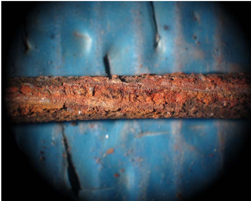
Figure 2b Steel Core Wire - Magnified View of Area with Surface Pitting Circuit D2L
