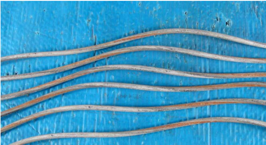
Figure 1b Outer Layer Aluminum Wires - Inner Surface Circuit D2L
