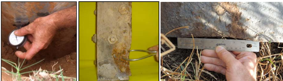
Figure 2-3: Damage Measurements, Pitting (L), Thinning (M), Edge Loss (R)
