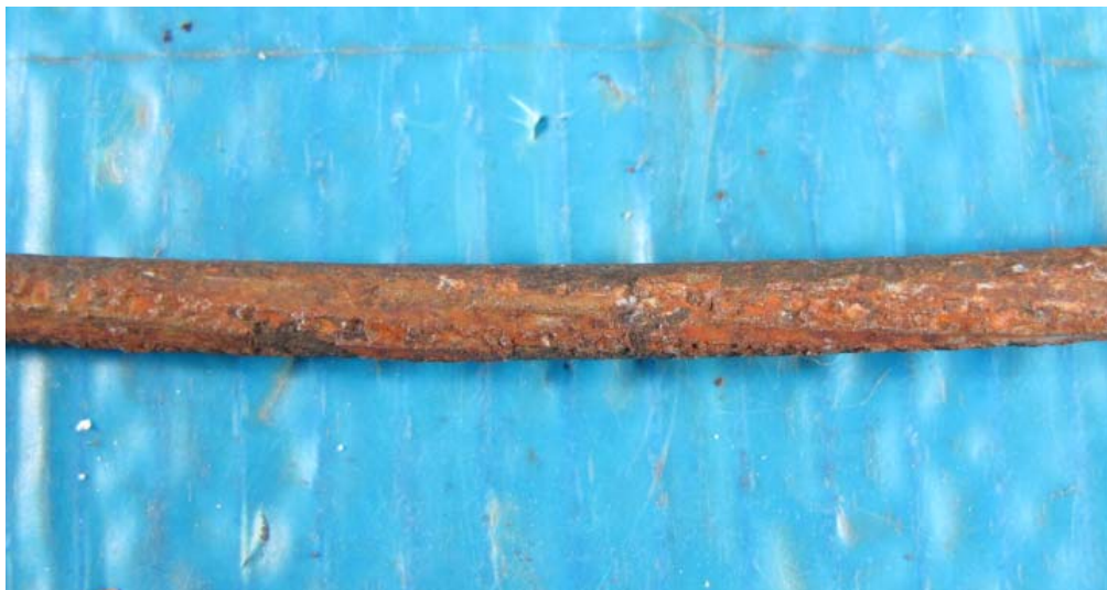
Figure 2a Steel Core Wire - Outside Surface Circuit D2L
