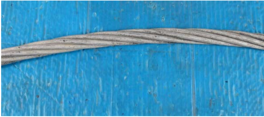
Figure 1a Outer Layer Aluminum Wires - Outer Surface (complete conductor) Circuit D2L
