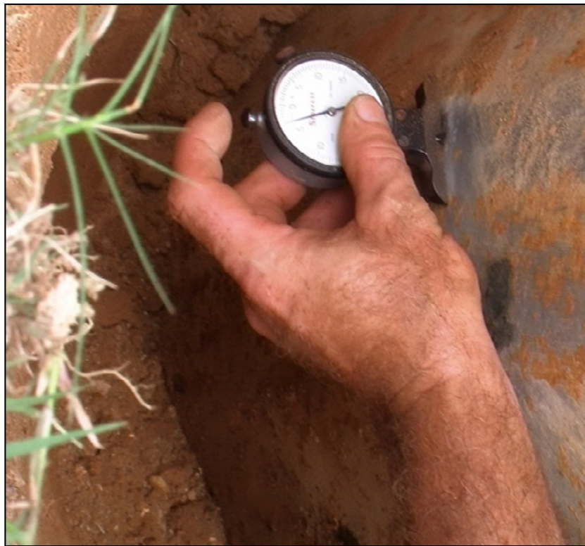
Figure 5-1: Dial Vernier Depth Gage with a Pointed Spindle
