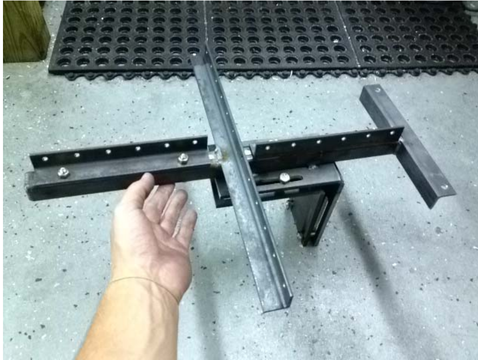
Figure 4-1: Coupon Rack Design for Attachment to the Structure
