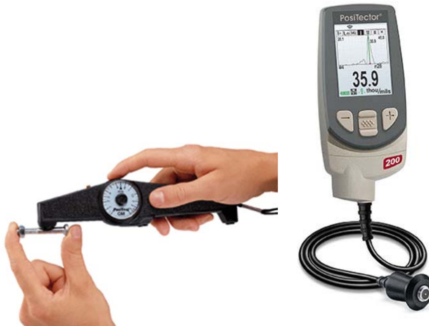
Figure 2-1 Magnetic Pulloff Gauge (L), and Ultrasonic Gauge (R)
