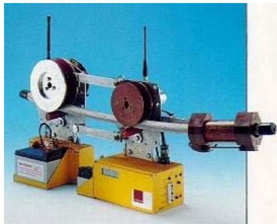
Figure 2: Cormon Overhead Line Corrosion Detector
