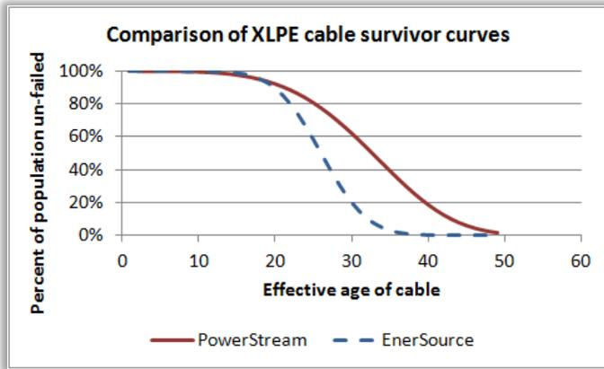
Comparison of survival curves for non-tree-retardant, direct buried XLPE cable used by PowerStream and Enersource.
