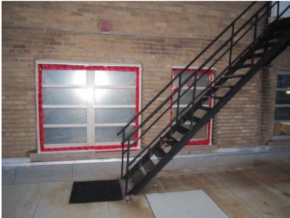
Photo 5. Exterior view of Window 2 and Window 3 bagged on the exterior (bagged in order to calculate extraneous leakage)
