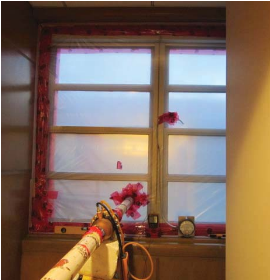
Photo 7. Interior view of Window 3 being tested for air leakage
