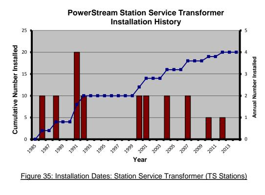
4 Figure 35 indicates that the station service transformers are widely dispersed in age, from four
