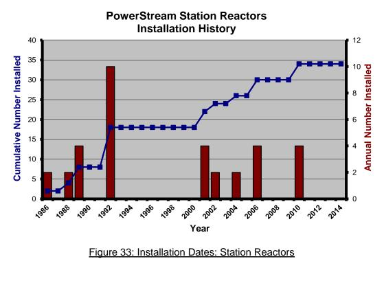
4 Figure 33 indicates that the station reactors are widely dispersed in age, from four to 28 years of age.
