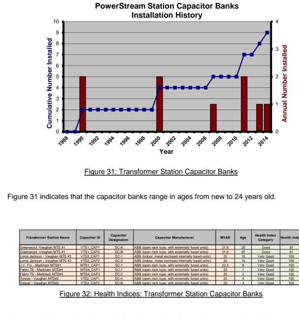
10 Figure 32 indicates that all capacitor banks are either in good or very good condition.
