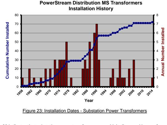
4 Figure 23 indicates that substation power transformers are widely dispersed in age, from new to 56 years of age.
