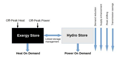
The exergy store accumulates both heat and exergy (which contributes the power) at times when they are plentiful and the store returns both the heat and the electrical benefits according to the fluctuations in demand. The demand reduction and the supply enhancement (and the reduction in transmission losses) have the same effect on the power grid as might be achieved by expanding the power generation capacity - but no new generators need to be built.
