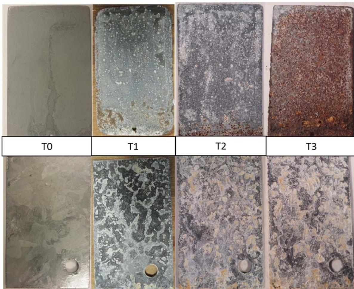
**Figure 30: Top: Galvatech coupon #4 as it is aged. Bottom: galvanized coupon #4 as it is aged**
