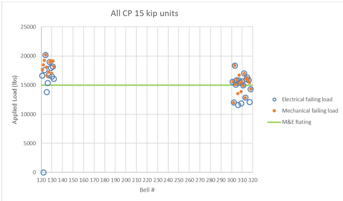
**Figure 5: M&E test results for insulator lot 4**
