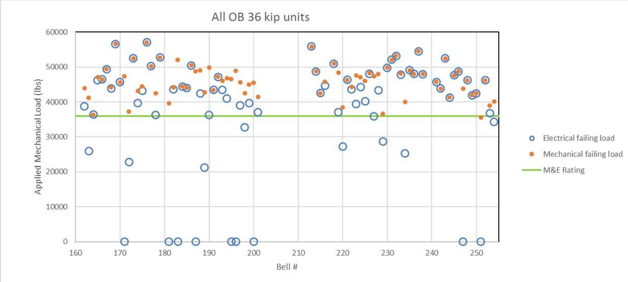
Figure 3: M&E test results for insulator lot 2
