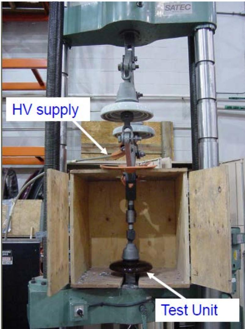
Figure A3: Insulator undergoing the M&E Test (test 3)
