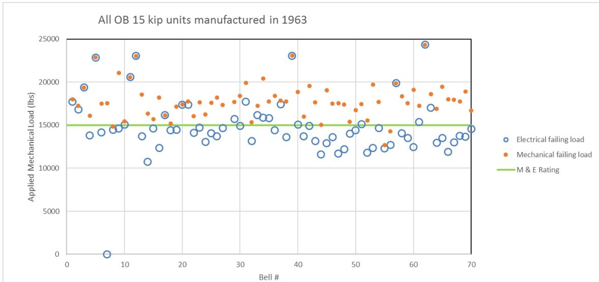
Figure 6: M&E test results for insulator lot 5
