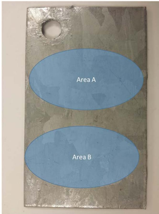
**Figure 26: Coating thickness measurements areas for all galvanized coupons.**
