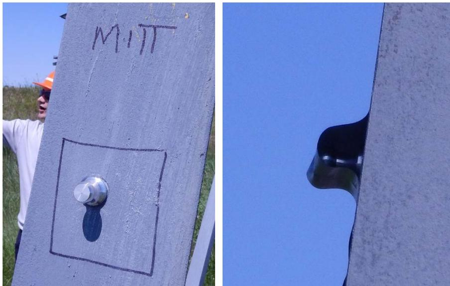
**Figure 32 Dollie Adhered to Lattice Surface (L); Tape Securing Dolly during Dry Time (R)**
