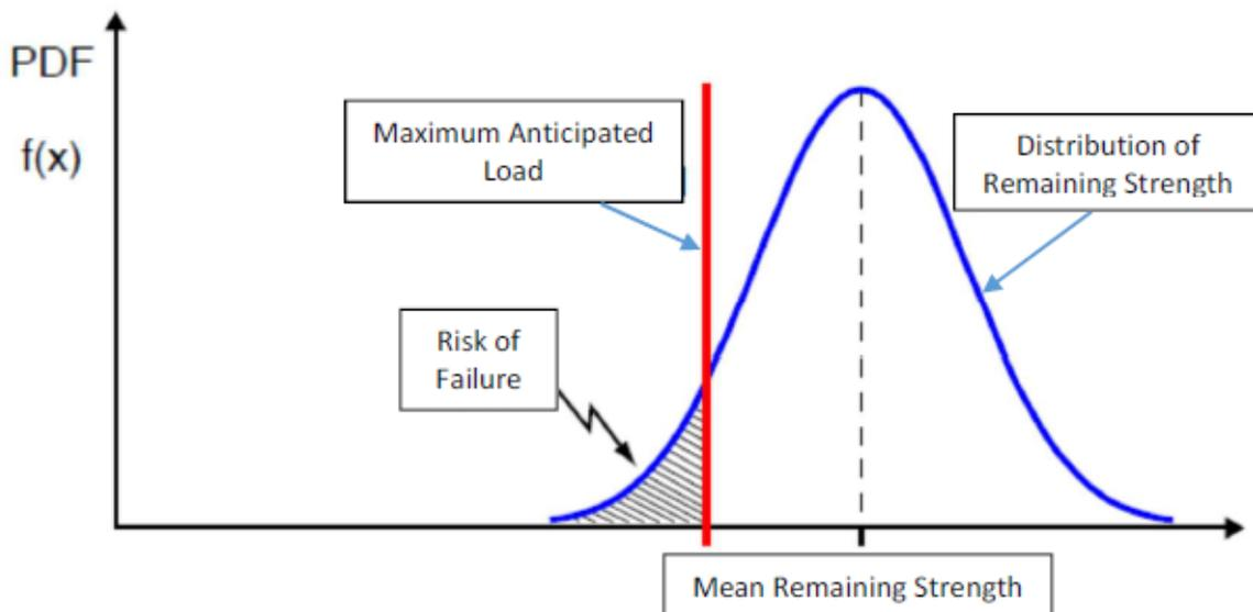
**Figure 11: Maximum applied load vs ultimate mechanical strength**
