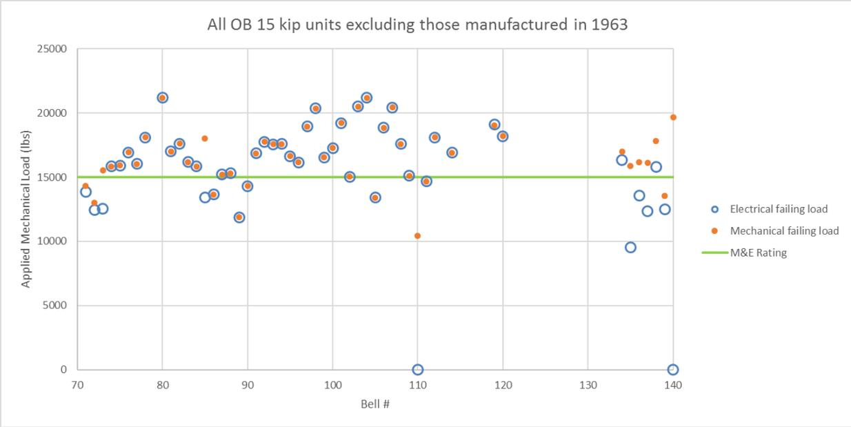
Figure 2: M&E test results for insulator lot 1
