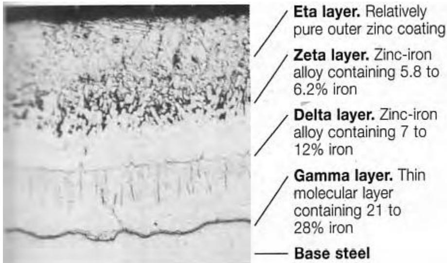
Figure 28: Zinc/Iron layers of galvanized steel
