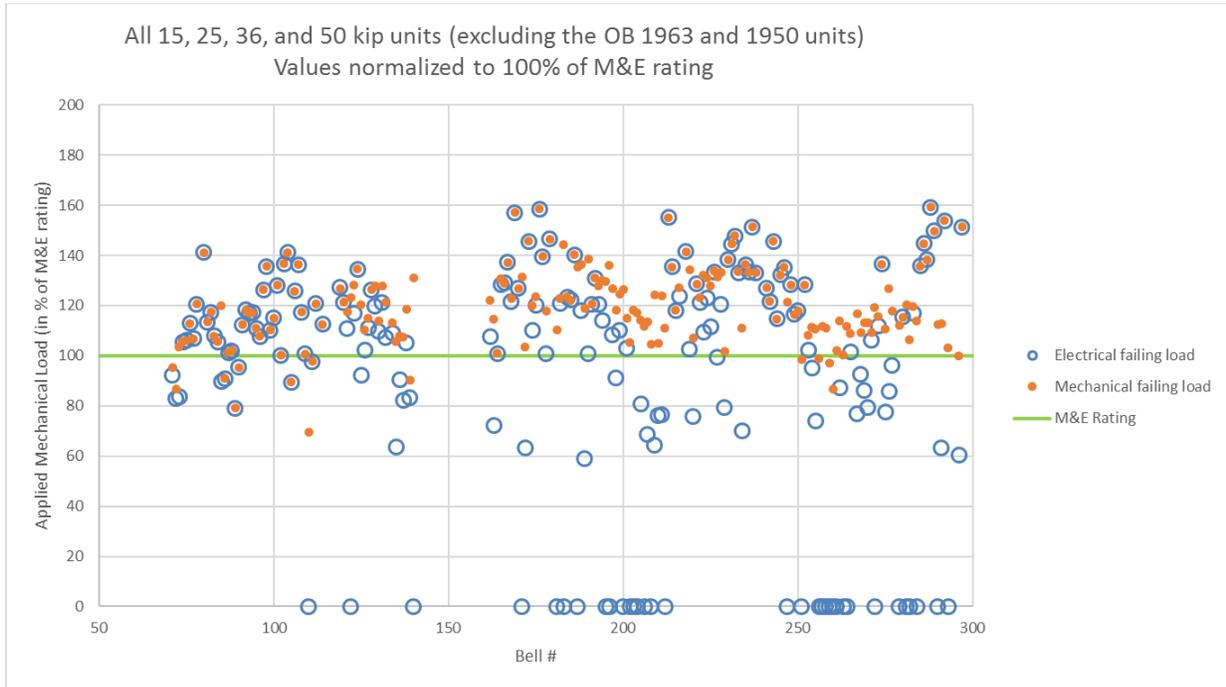
**Figure 1: Normalized M&E test results for insulator lots 1, 2, 3, 4, and 7 combined**
