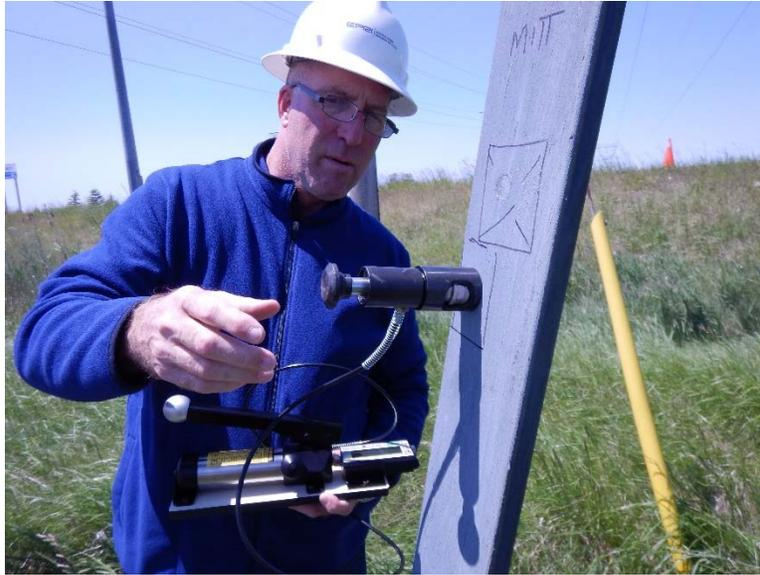
**Figure 33 Pull Off Adhesion Test using a Hydraulic Ram with Digital Readout**
