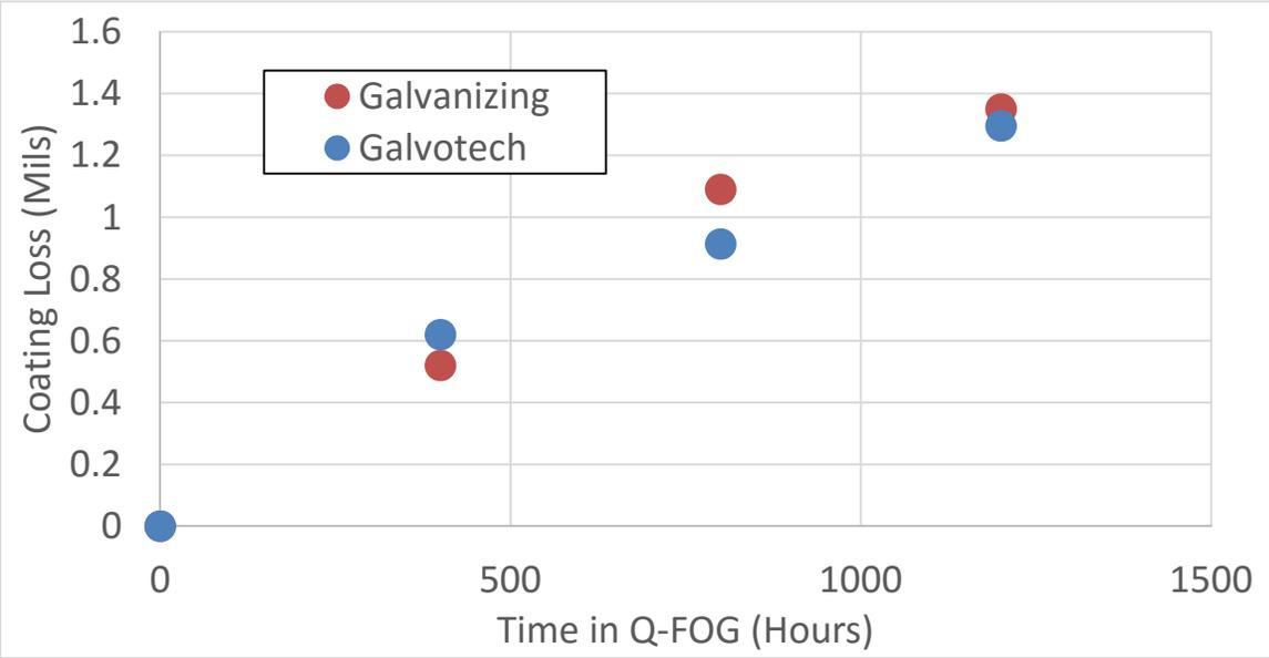
**Figure 29: Coatings Degradation Rate**
