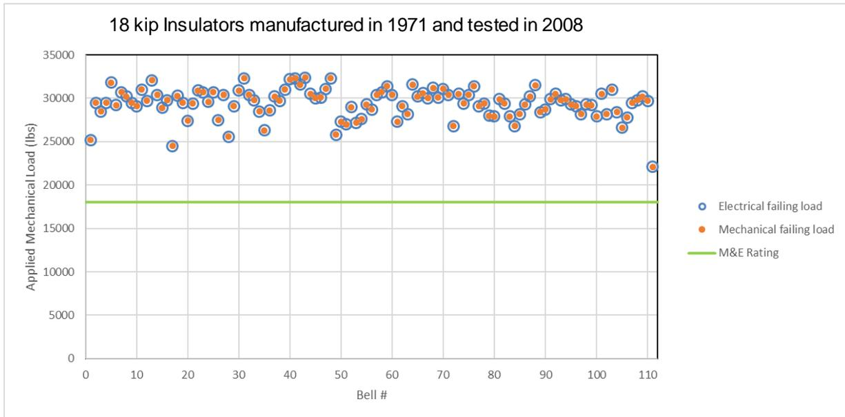
**Figure 8: M&E test results for 18 kip insulators on Manitoba Hydro's transmission system**
