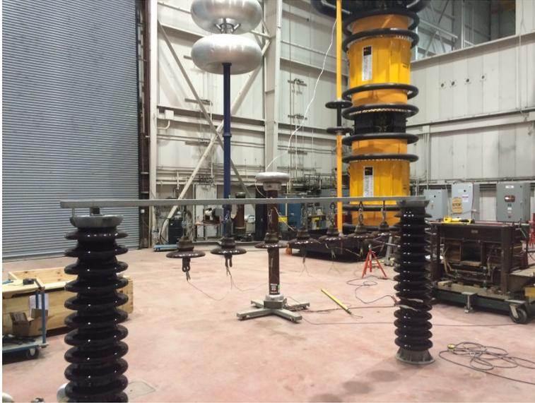
**Figure A2: Insulators undergoing the ac withstand test (test 2)**
