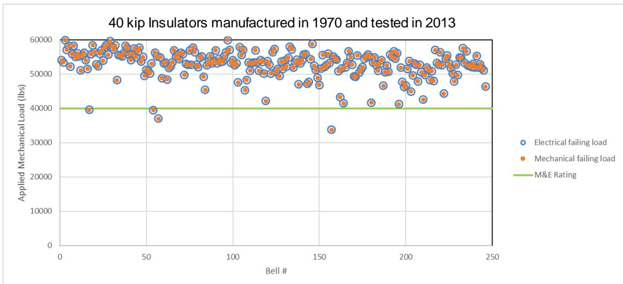
**Figure 9: M&E test results for 40 kip insulators from EPRI's data base**
