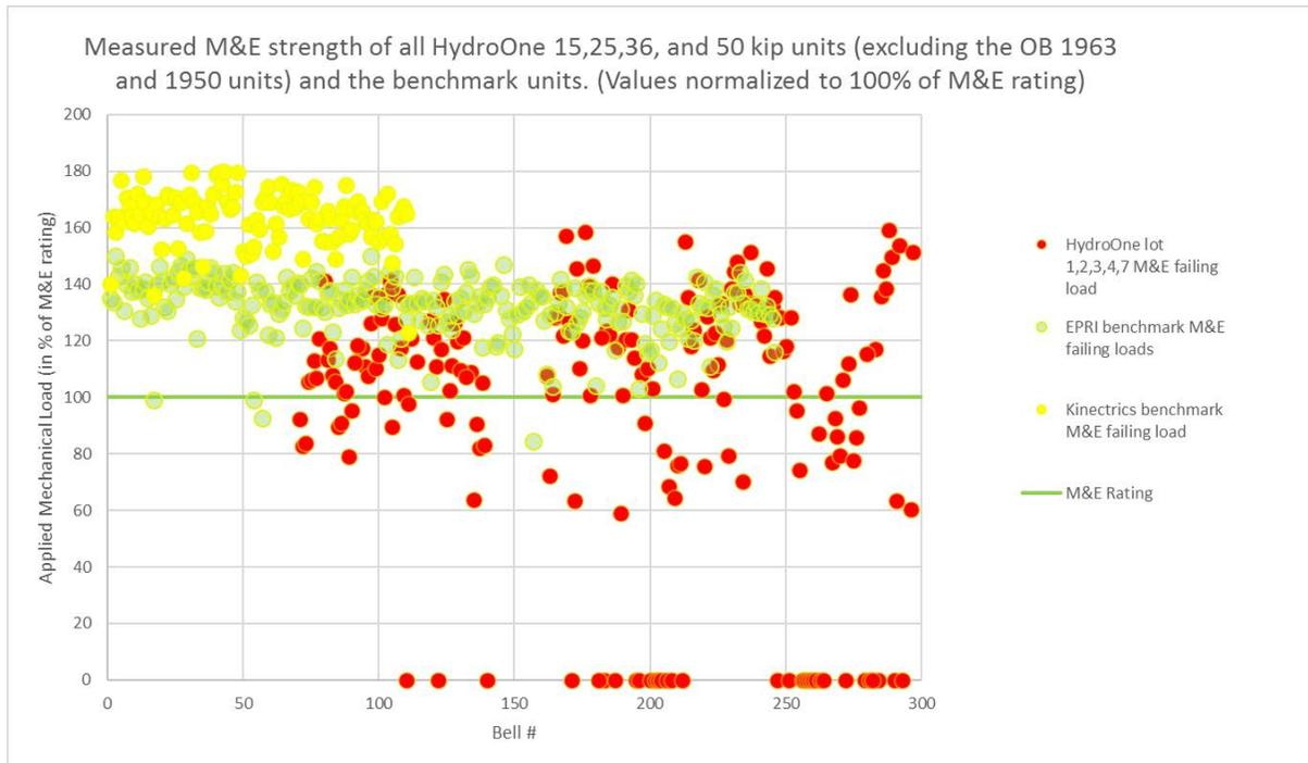
**Figure 10: M&E test results normalized to 100% of rating for HydroOne combined lot 1,2,3,4 and 7 insulators plotted together with the results from the benchmark insulators**
