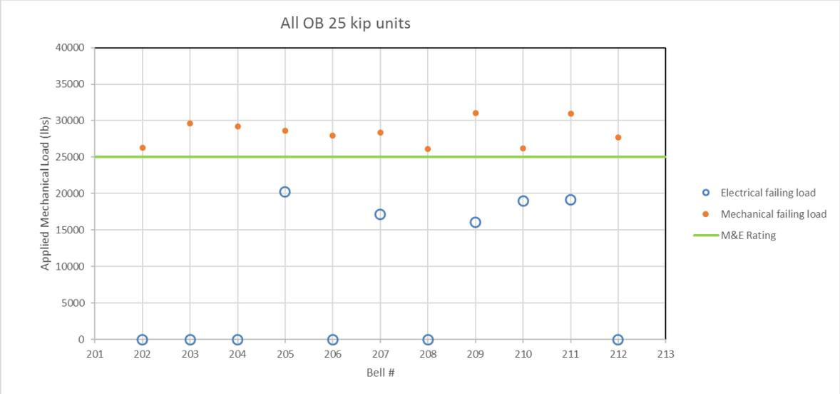
**Figure 8: M&E test results for insulator lot 7**
