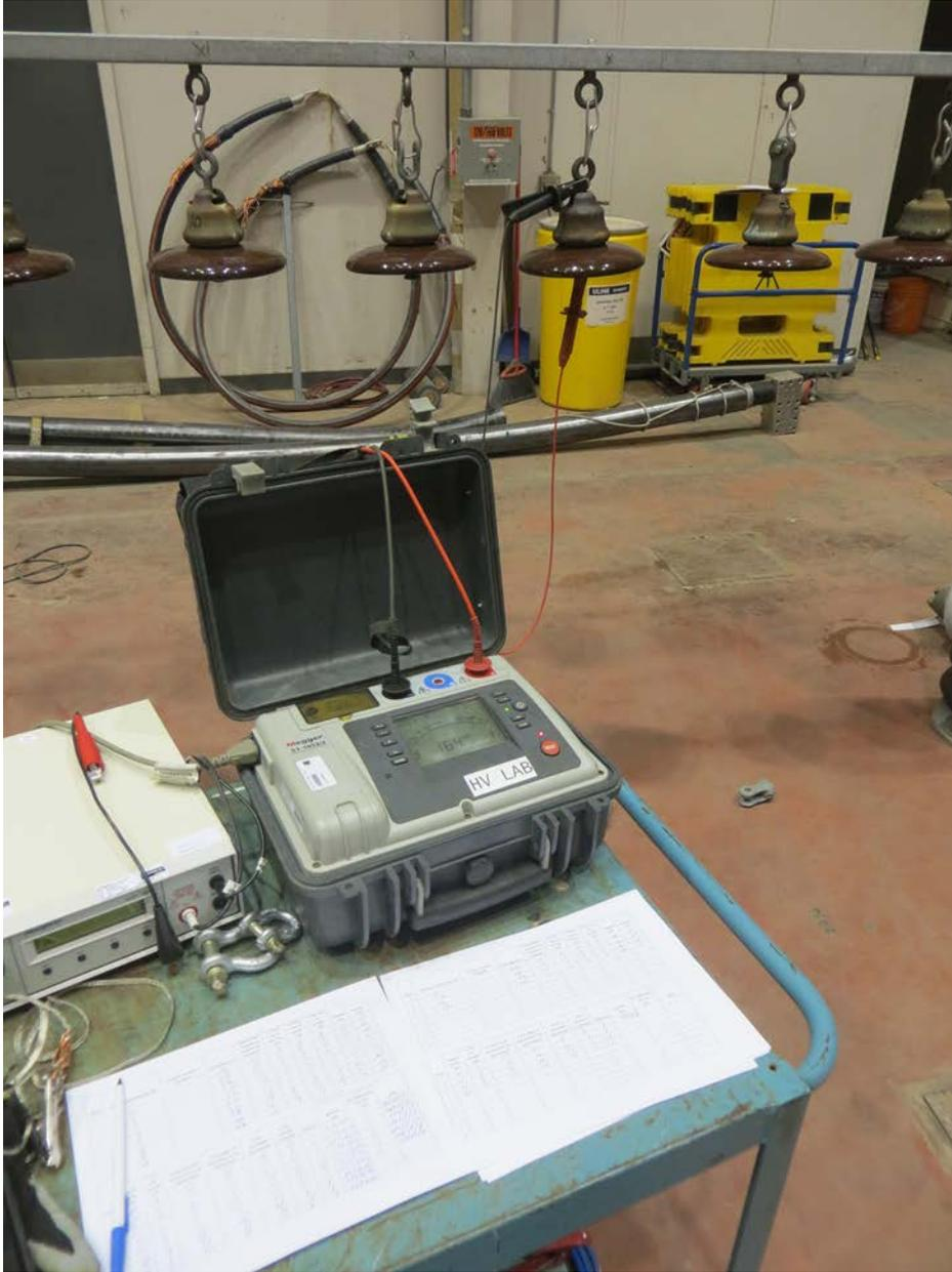
**Figure A1: Insulators undergoing the Megger test (test 1)**
