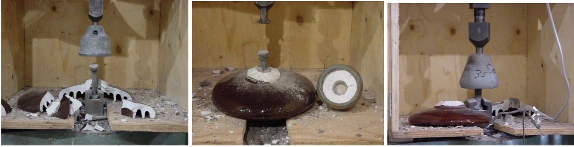
**Figure A4: Typical modes of failure observed during M&E testing**
