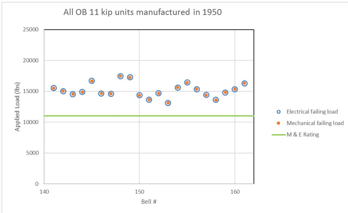
Figure 7: M&E test results for insulator lot 6
