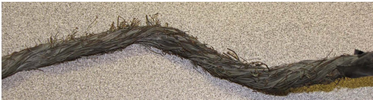
Figure 8-5 - Frayed Arrester Bond Wire
