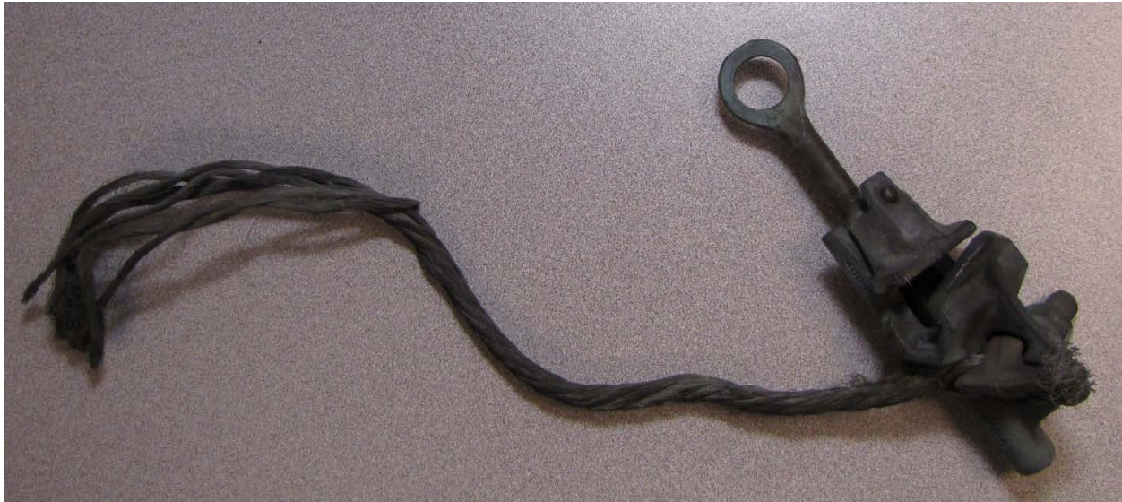
Figure 8-4 - Failed Arrester Bond Wire
