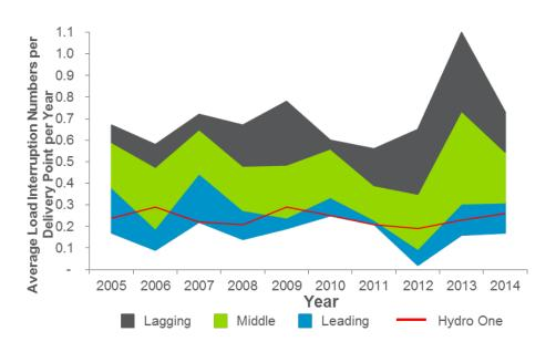
Figure 20. Sustained T-SAIFI-mc Comparison by the CEA
