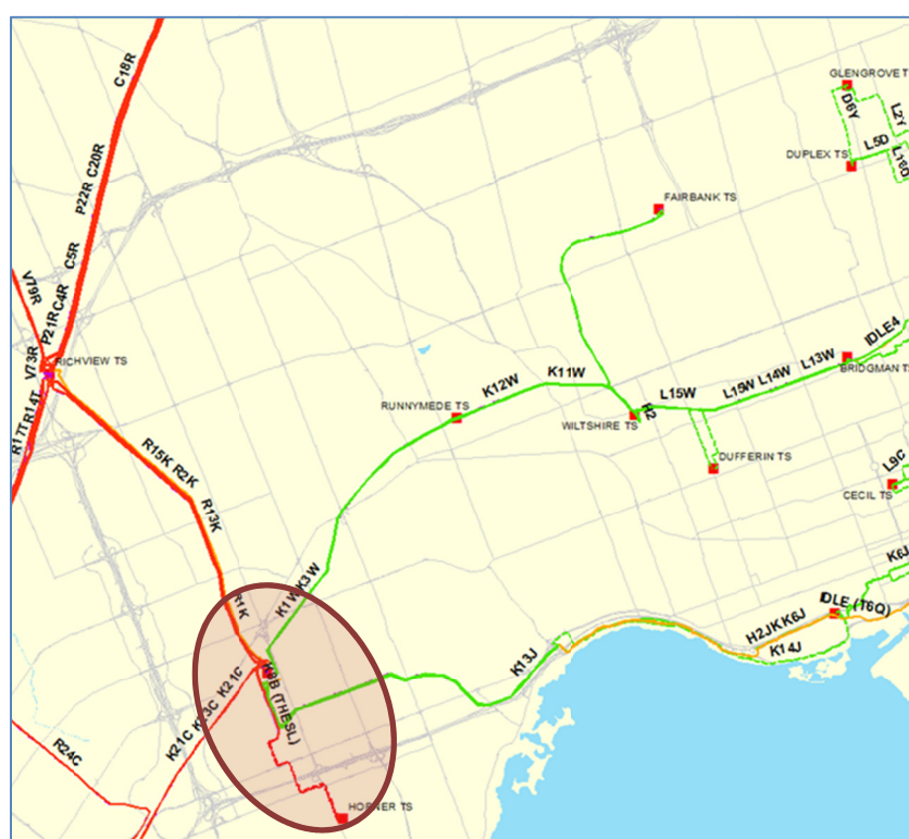
Figure 7-2 Horner TS and Manby TS Supply Area
