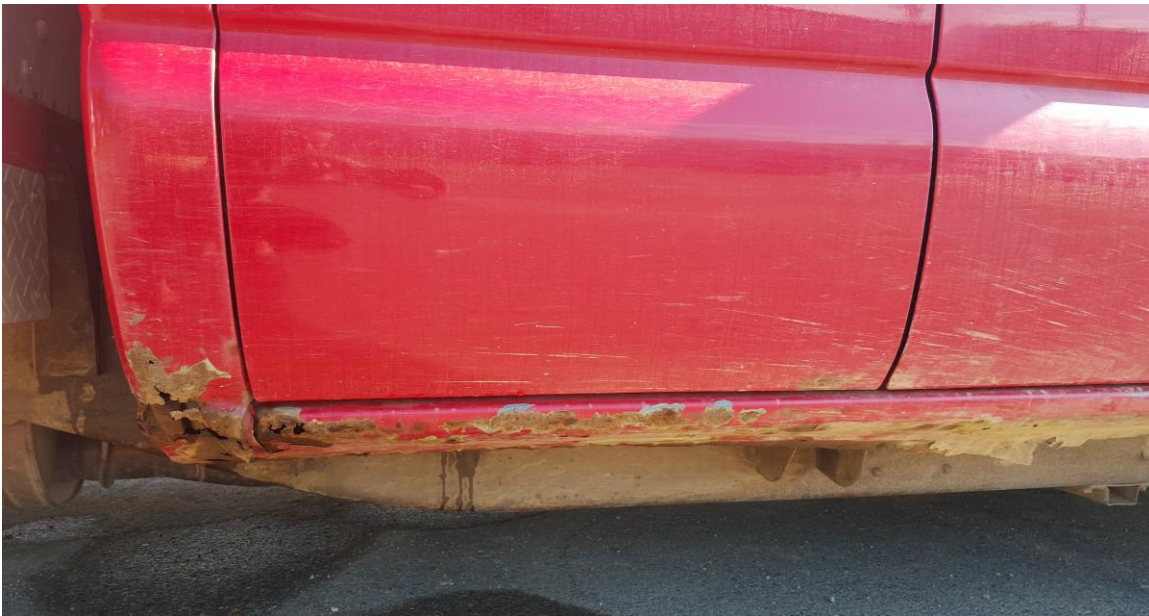
Visual showing some of the rust and deterioration of the body.
