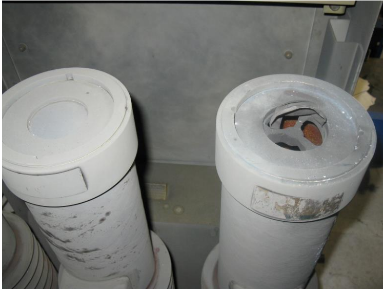
Figure 15 - Image of Catastrophic Failure of Richmond Hill TS#1 Circuit Breaker
