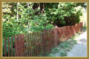
Plate 5. Example of a wood lath snow fencing used to exclude turtles (photo credit: Karine Beriault).
