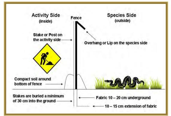
Figure 1. A side view of a basic exclusion fence including an overhang or flexible lip to deter animals from climbing or jumping over the fence. Placement of the stake on the Activity Side or on the inside of excluded area is also illustrated. This is particularly important for snake species which may use the stakes to maneuver over the fence.
