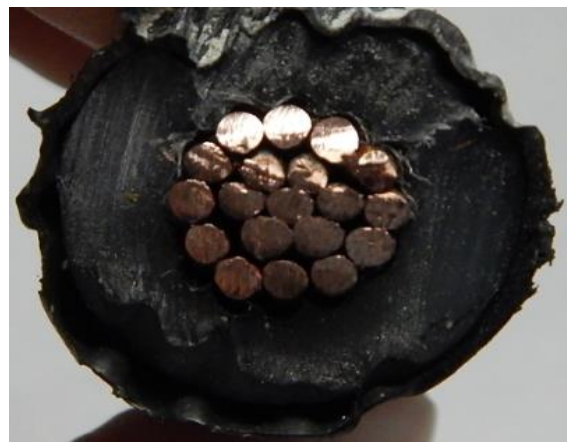
Figure 7: Stranded Conductor - 1/0 and Main feeder – CU (16.9% failure rate)
