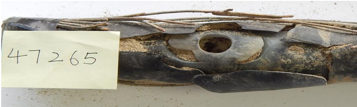
Figure 5: Direct buried conductors without a jacket, solid or stranded - 1/0 & main feeder
