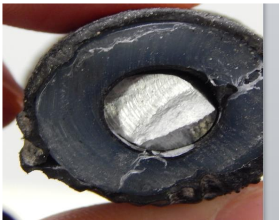
Figure 6: Solid Conductor - 1/0 – AL (62.1% failure rate)
