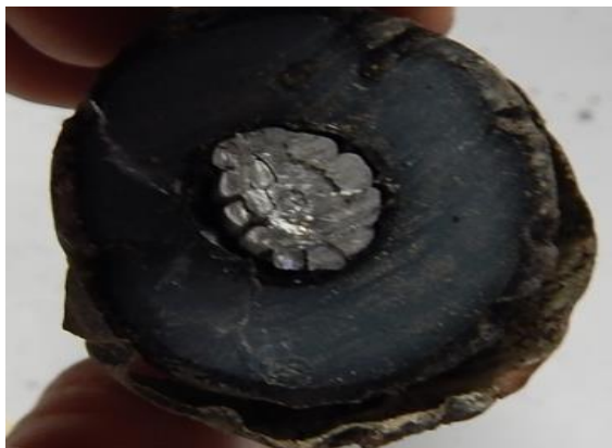
Figure 8: Stranded Conductor - 1/0 – AL (1.6% failure rate)
