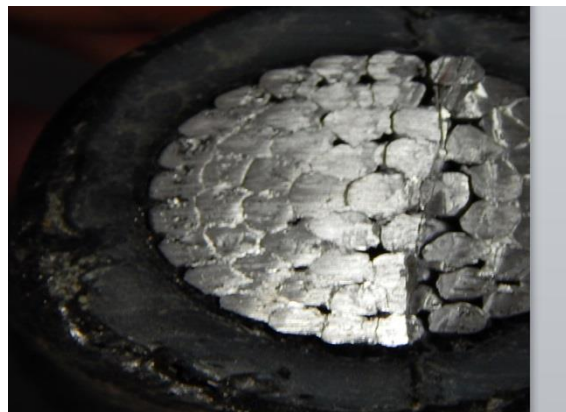
Figure 9: Stranded Conductor - Main feeder – AL (19.4% failure rate)
