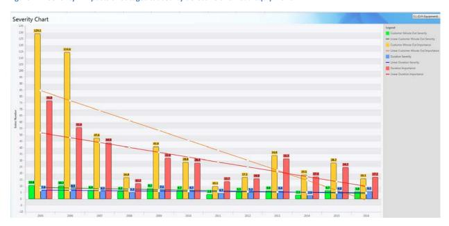
Figure 2-3: Severity - Impacts of outages caused by defective underground equipment
