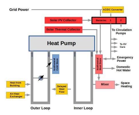
Exergy stores provide thermal storage in two ways: via the heat stored in the core and via the wave of heat that flows out of the core and that reaches the outer ring by the winter, at which time the heat pump returns the heat to the core, stabilizing its temperature. The electricity storage takes many forms:
