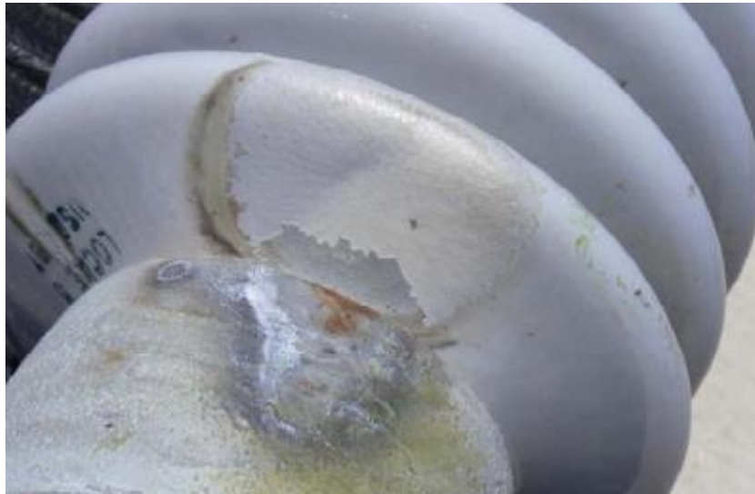
Figure 10: Close-up of Damaged Porcelain Insulator Showing Tracking
