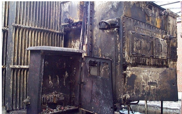
Figure 23: Failed Power Transformer
