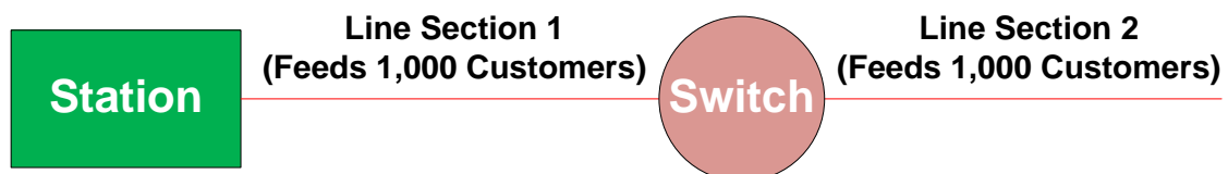
Figure 9: Example of Overhead Switch Impact on System Reliability
