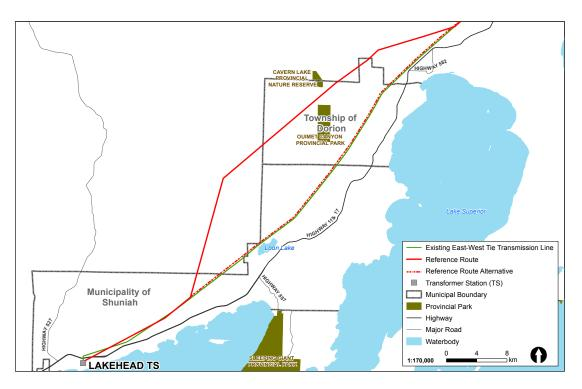
The Dorion reference route alternative section follows the existing East-West Tie transmission line.
