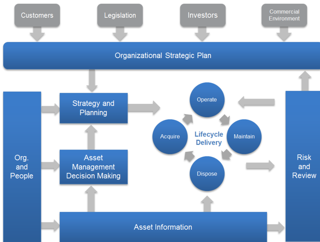
Figure 4.1.1: Asset Management – an anatomy, Version 3, page 16, Figure 3: The IAM’s Conceptual Asset Management Model, theIAM.org
