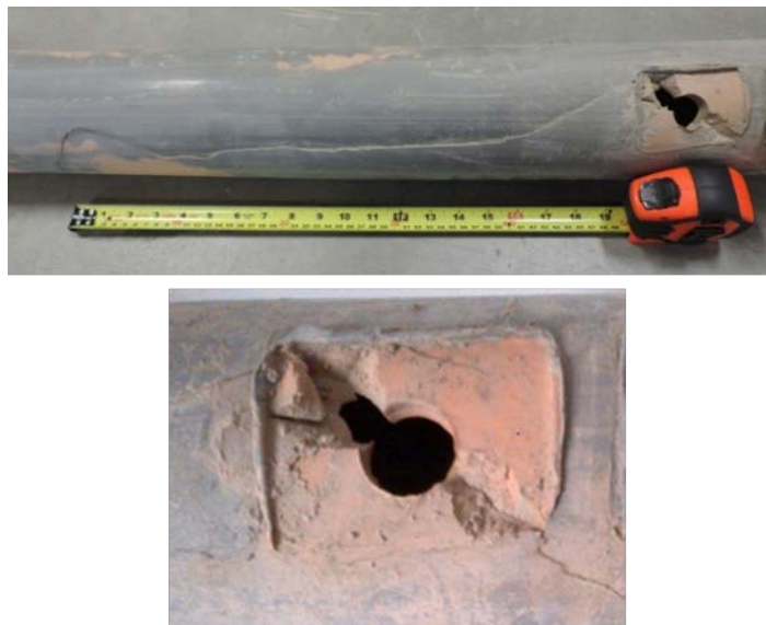
Figure 5.2-33: Rapid Crack Propagation on Aldyl A Pipe from Saddle Tee Fusion (Mississauga, ON)
