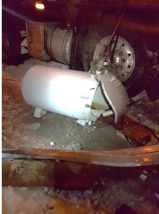
1           **Figure 9: Distribution Transformer Leaking Oil After Vehicle Impact with Pole**
