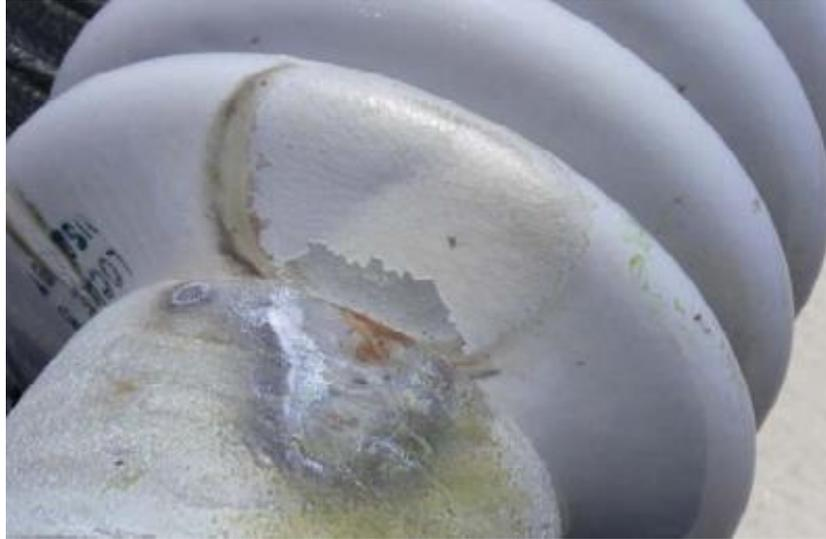
**Figure 10: Close-up of Damaged Porcelain Insulator Showing Tracking**
