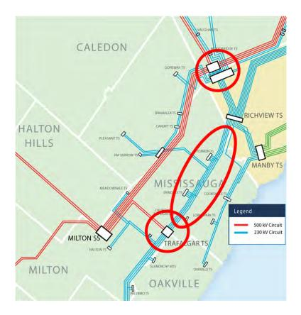
The two primary factors driving the overloads on the 500-230 kV transformers and the Trafalgar to Richview 230 kV lines are load growth in the GTA and changes in generation patterns across Ontario. While all growth within the GTA has some impact on the bulk system, growth within West GTA (the municipalities of Mississauga, Oakville, Milton, Halton Hills, Brampton and Caledon) has the greatest contribution due to proximity to the affected bulk facilities.
