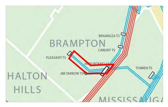
Based on the assessment carried out as part of the NW GTA IRRP, the maximum carrying capacity of the transmission line to Pleasant TS is approximately 417 MW. Since the need is dependent on the total loading of all three step-down facilities supplied by this line, the actual need date is sensitive to assumptions about the net growth rate. The table below summarizes forecast need dates under the Expected and Higher Growth scenarios:
