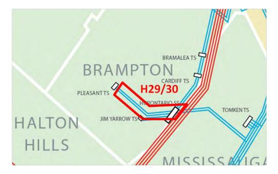
Two transmission-based solutions are considered below: upgrading the existing H29/30 circuits to a higher rating and advancing the construction of a new transmission supply path into the area.
