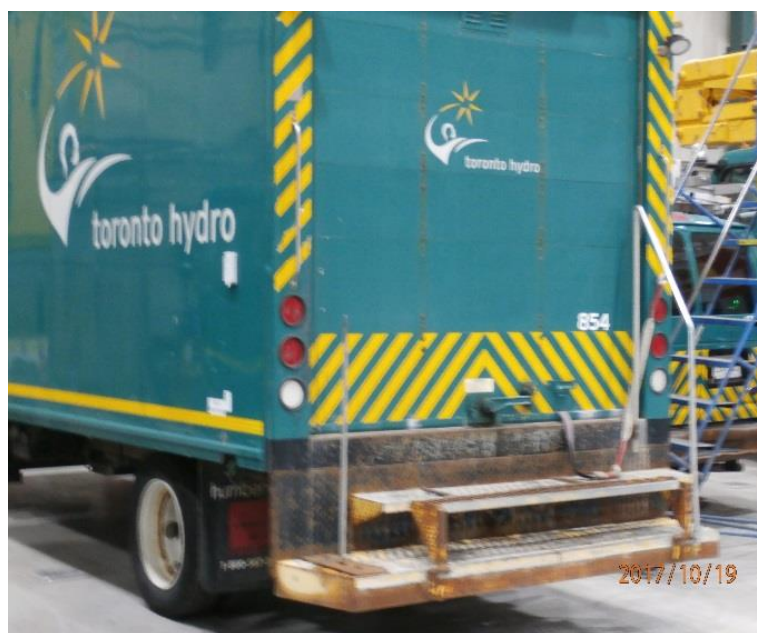
Figure 2: Corrosion on Cube Van Steps
