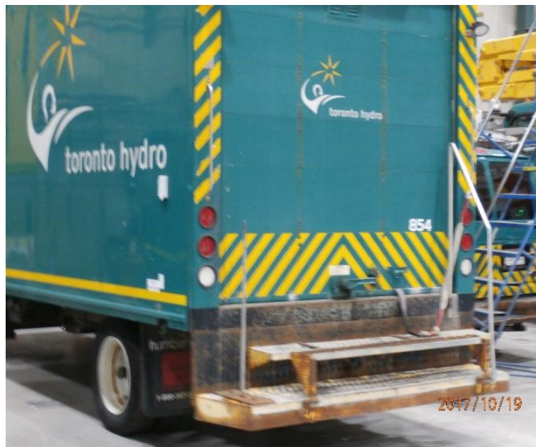
Figure 2: Corrosion on Cube Van Steps
