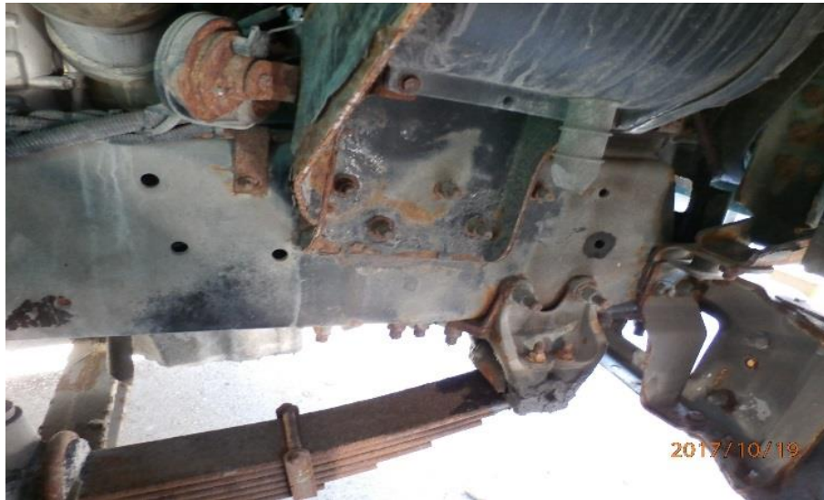
5 Figure 3: Underbody Corrosion on Bucket Truck
