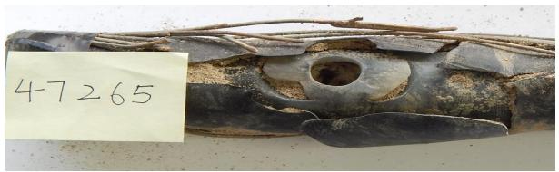
Figure 5: Direct buried conductors without a jacket, solid or stranded - 1/0 & main feeder
