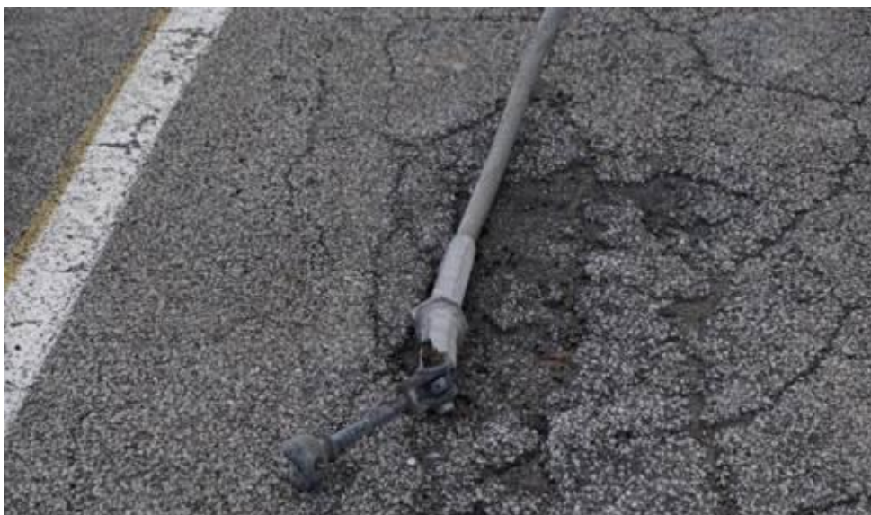
Figure 5 - Damage from a fallen conductor
