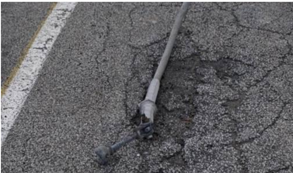
Figure 5 - Damage from a fallen conductor
