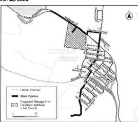
Township of Terrace Bay: Construction of 5 kilometres of main pipeline along the TransCanada Highway, Mill Road, and an unnamed street and 13 kilometres of lateral lines extending from the main line, as shown in the map below
