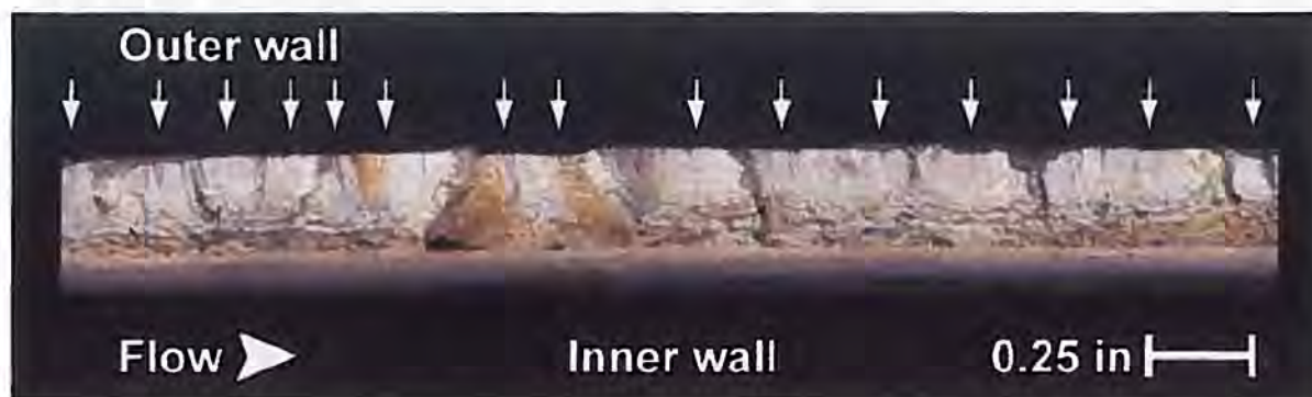
Figure 13. Curving arrest lines of preexisting cracks along the upper fracture face shown after cleaning to remove oxides. White arrows indicate multiple origin areas of preexisting cracks.
