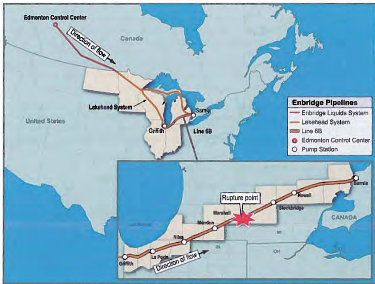
Figure 1. Enbridge's Liquids System and the 1,900-mile Lakehead System (the U.S. portion). Inset shows Line 6B, the 293-mile extension from Griffith to Samia installed in 1969.
