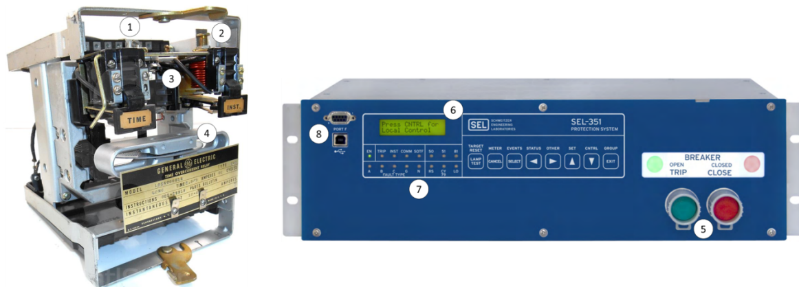
Figure 6.17 – Station Protective Relays
