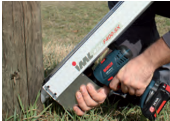
Figure 8 – Pole Testing Using Resistograph Drill
