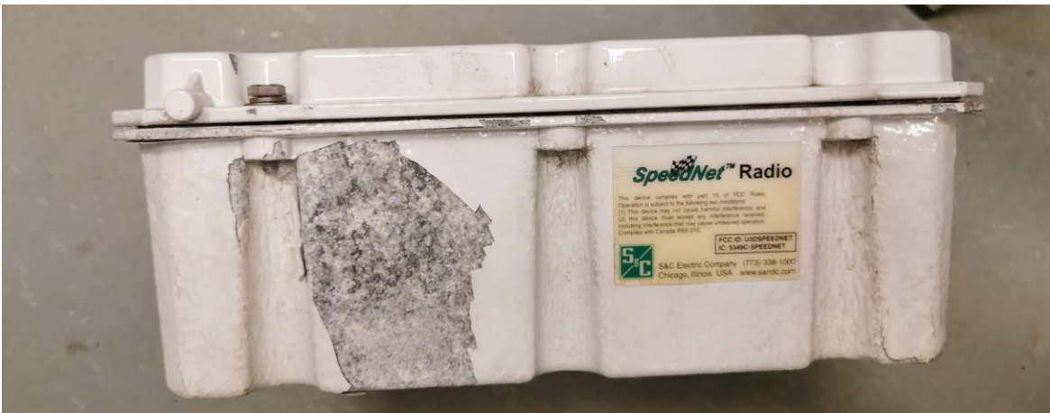
Figure 70- Example of a failed Radio Communication Box that failed to communicate due to moisture ingress (Outside)
