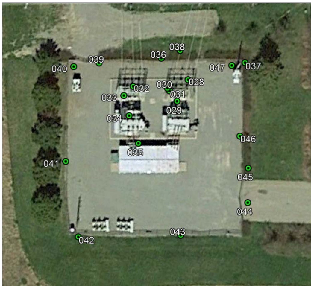
Figure 9-1: Integrity Test Locations at MS 13
