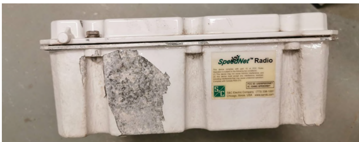
Figure 70- Example of a failed Radio Communication Box that failed to communicate due to moisture ingress (Outside)
