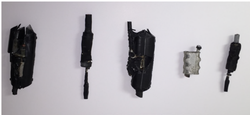
Figure 65: Photo of bi-metallic corrosion
