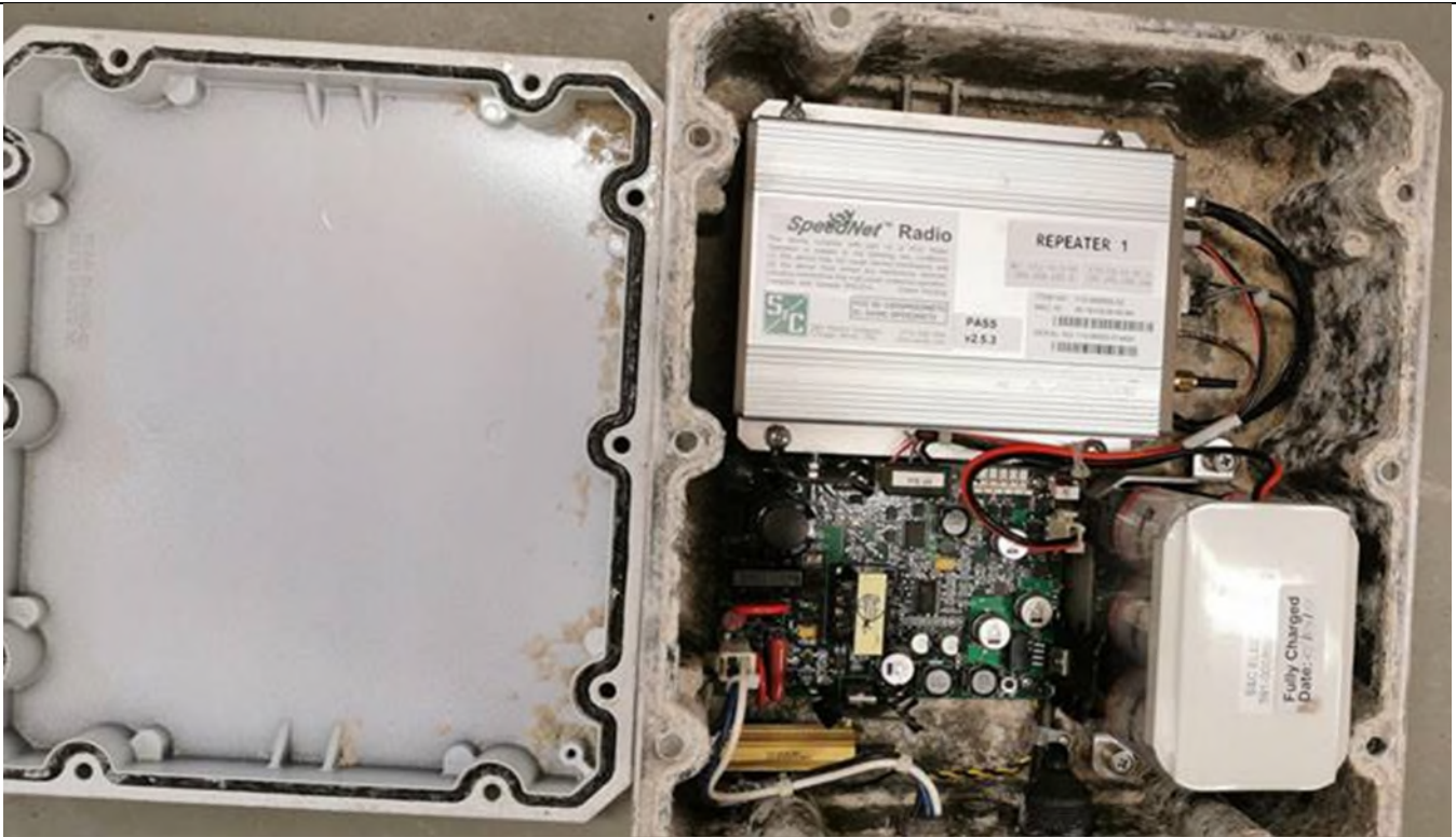
Figure 71- Example of a failed Radio Communication Box that failed to communicate due to water ingress (Inside)
