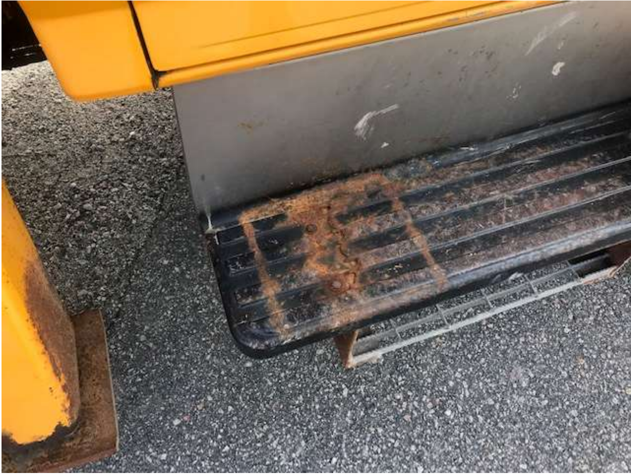
Rust on Running Board and Outrigger
