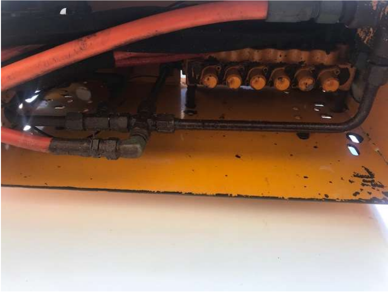
Some of the Hydraulic Hoses that need to be replaced
