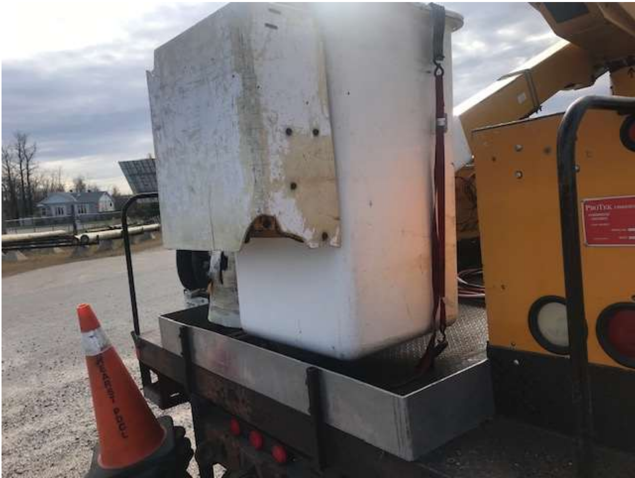
Bucket Wear and Tear
