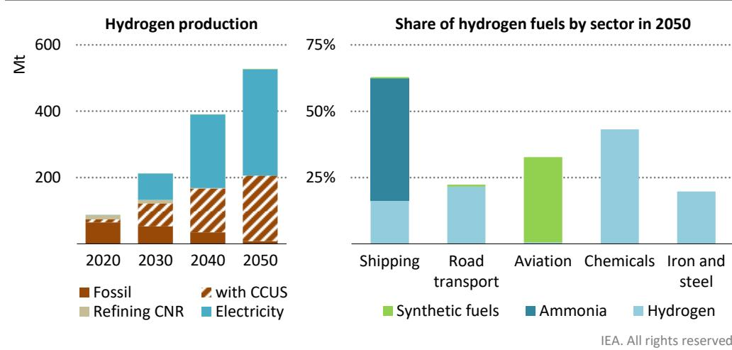
**Hydrogen production jumps sixfold by 2050, driven by water electrolysis and natural gas with CCUS, to meet rising demand in shipping, road transport and heavy industry**
