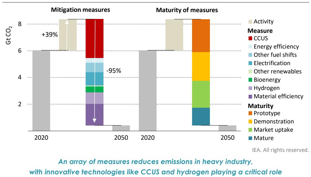
Hydrogen and CCUS technologies together contribute around 50% of the emissions reductions in heavy industry in 2050 in the NZE. These technologies enable the provision of large amounts of high-temperature heat, which in many cases cannot be easily provided by electricity with current technologies, and help to reduce process emissions from the chemical reactions inherent in some industrial production. Bioenergy also makes a contribution in a wide array of industrial applications.
