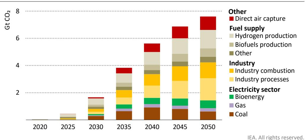
By 2050, 7.6 Gt of CO<sub>2</sub> is captured per year from a diverse range of sources. A total of 2.4 Gt CO<sub>2</sub> is captured from bioenergy use and DAC, of which 1.9 Gt CO<sub>2</sub> is permanently stored.
