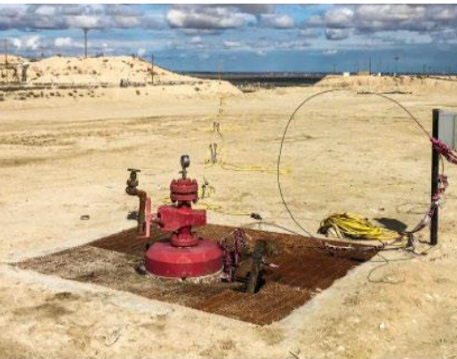
Successful field operation test on an 800-ft deep oil well at Chevron's Cymric Oil field
