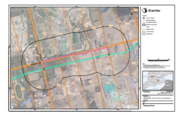
The Sarnia Products Pipeline is a 74.23 km long, NPS 12 petroleum products transportation pipeline, connecting Imperial Oil's Waterdown Pump Station and Nanticoke Pump Station.
